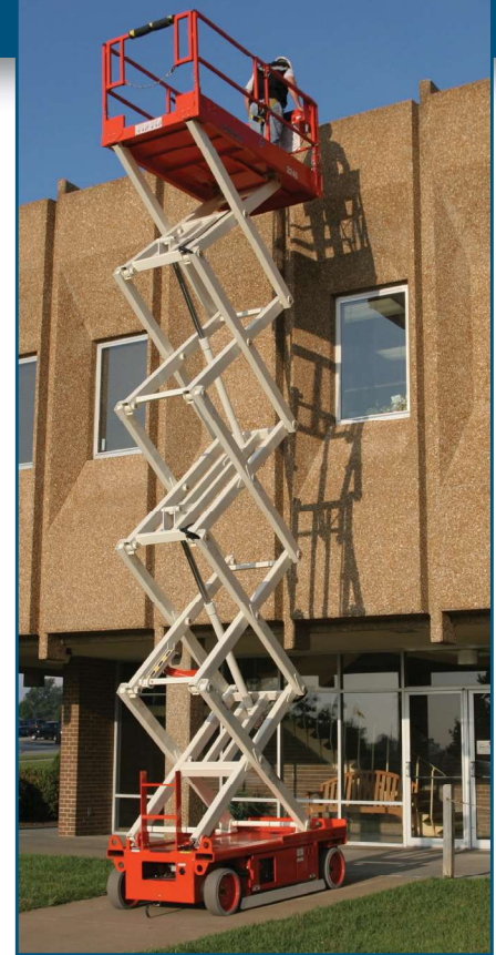
Snorkel states the only time a harness is required on a scissor is when a particular site requires it or if there are specific local regulations.
