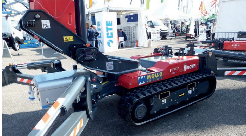
Hinowa's LL33.17 PHS is available in a new version: a Lithium and diesel version and a Lithium-only version has been available previously.
